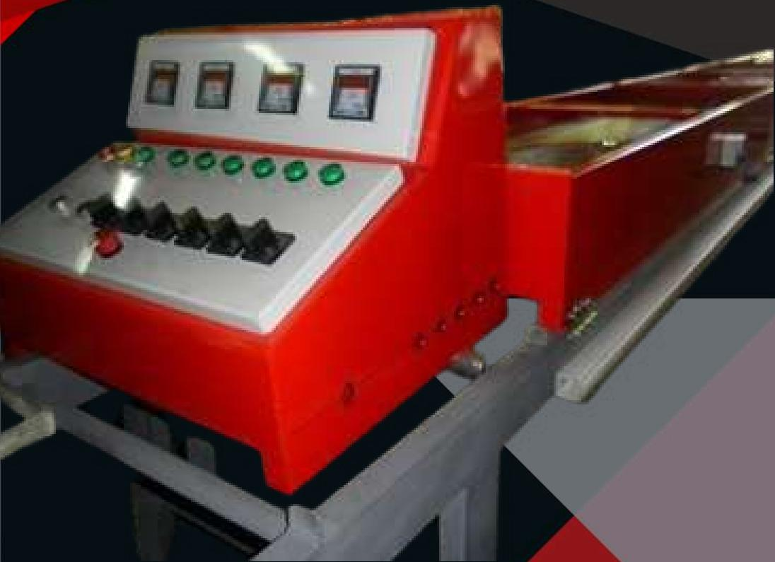
This is a C-type semi-automatic cube sugar machine. The machine produces cube sugar from granulated sugar, but manual labor is required for packaging. In R-type fully automatic machines, the packaging unit is automatic. Its 24-hour production capacity ranges between 6 and 7 tons.
