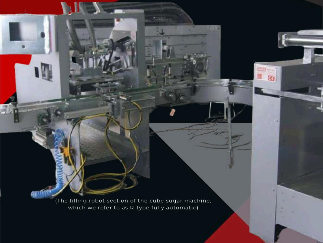
(The filling robot section of the cube sugar machine,
