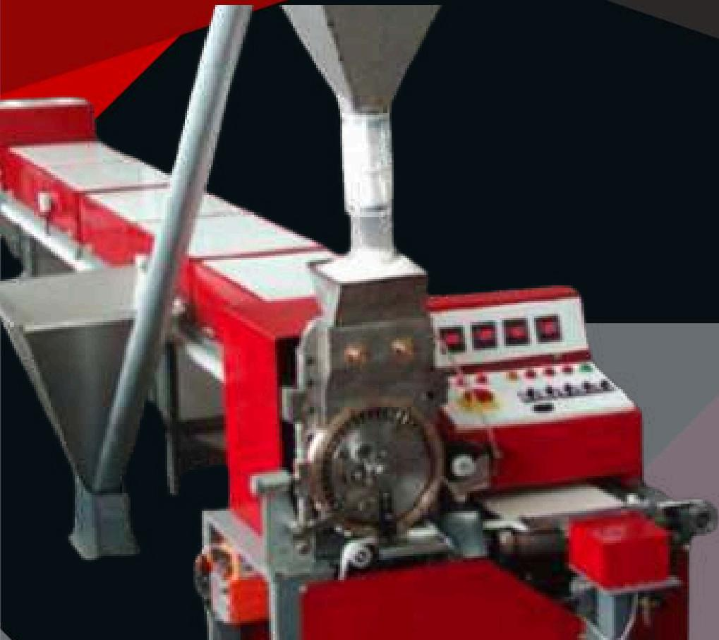
This is a C-type semi-automatic cube sugar machine. The machine produces cube sugar from granulated sugar, but manual labor is required for packaging. In R-type fully automatic machines, the packaging unit is automatic. Its 24-hour production capacity ranges between 6 and 7 tons.
