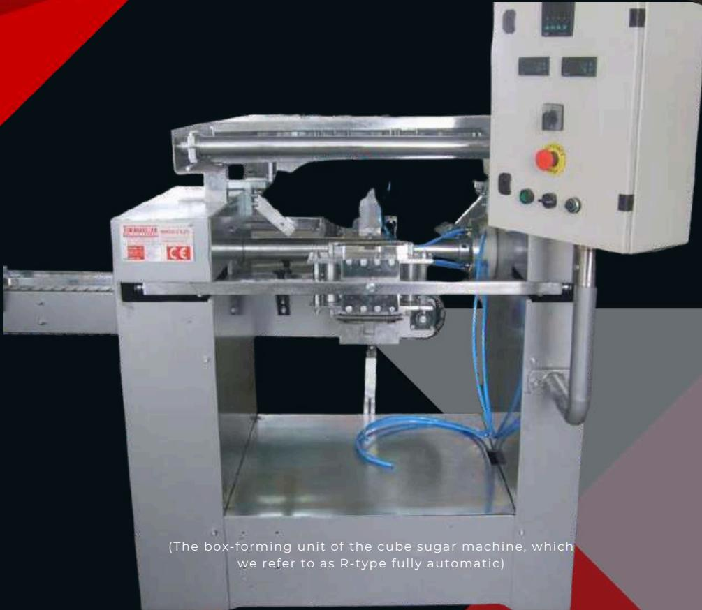
(The box-forming unit of the cube sugar machine, which we refer to as R-type fully automatic)
