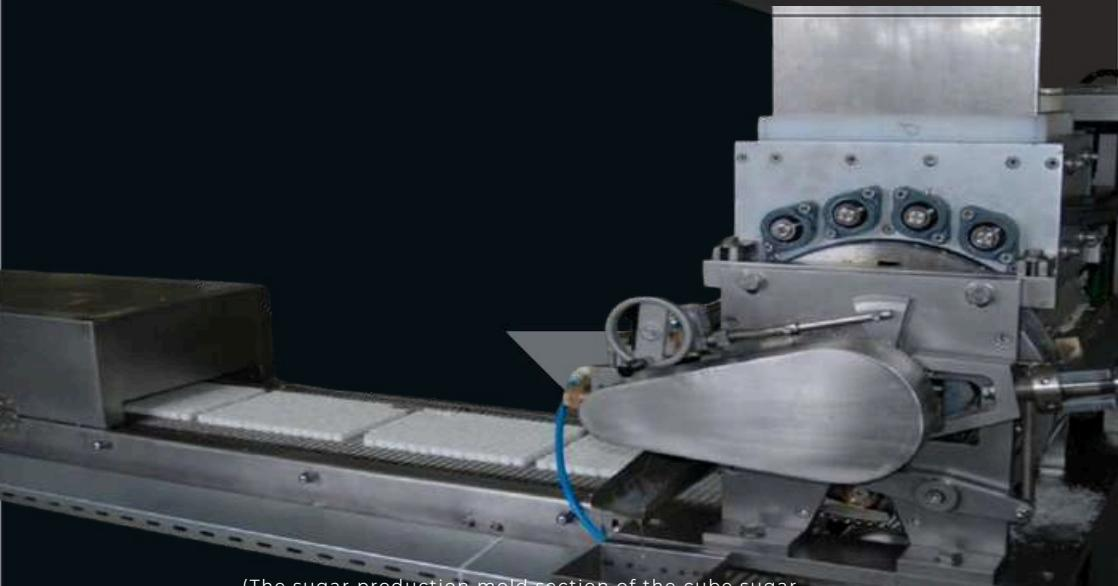
(The sugar production mold section of the cube sugar machine, which we refer to as R-type fully automatic)
