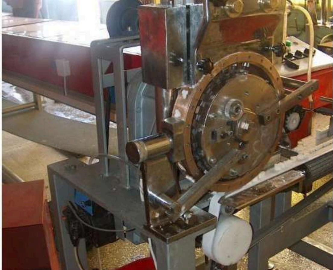
This is a C-type semi-automatic cube sugar machine. The machine produces cube sugar from granulated sugar, but manual labor is required for packaging. In R-type fully automatic machines, the packaging unit is automatic. Its 24-hour production capacity ranges between 6 and 7 tons.
